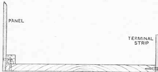
Fig. 11.—Method of securing panel and baseboard.
