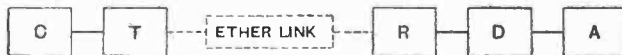
Fig. 1.—Showing the fundamental arrangements for distant control. C=actual control; T=generator of ether waves; R=receiver of ether waves; D=detector of ether waves; A=apparatus to be controlled.
