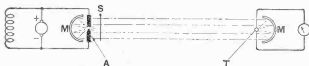
Fig. 6.—Arrangement of apparatus for heat-ray control.
