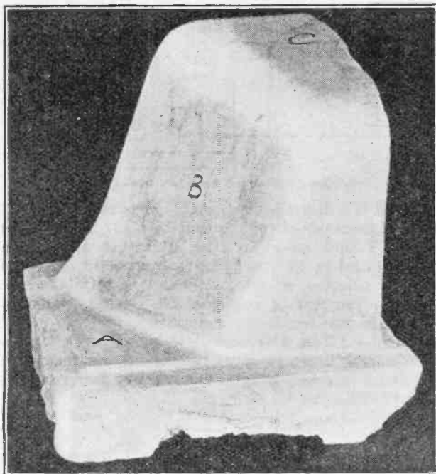
Fig. 6.—Model showing the areas into which the characteristic surface may be subdivided. A=zero anode current plane; B=useful working surface; C=saturation area.
