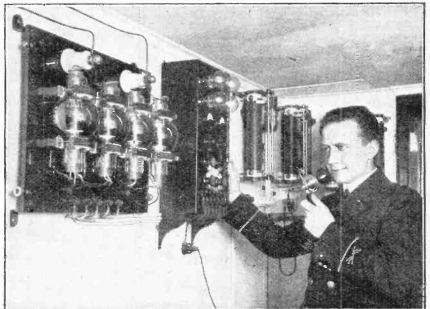
BROADCASTING FROM A SHIP. Part of the wireless telephony installation on board the Swedish motorship "Gripsholm," from which the President of the Swedish-American line recently delivered an address. The speech was picked up in Sweden and re-broadcast throughout the country. The microphone is connected to a two-stage push pull amplifier and the four modulator valves are seen on the left.
